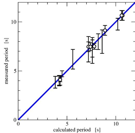
FIG. 7. (Color online) Correlation plot of the theoretical [see Eq. (1)] and measured periods for each experiment. White symbols denote the control results with the two-layer setup, the rest is for the three-layer experiments. Error bars are estimated from the half-width of the main Fourier peak shown in Fig. 6(b).
