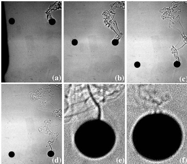
FIG. 1. Shadowgraph images over the first period of motion of a sphere [diameter  $d=14.6$  mm, ball density  $\rho_p=1.025(8)$  g/cm<sup>3</sup>,  $N=0.86 \pm 0.01$  1/s,  $(z_0 - z_{eq})/d=22.0$ , where the initial height was  $z_0=38.0$  cm]. The times after release are (a) 4 s, (b) 6.4 s, (c) 10 s, (d) 16 s, (e) 22 s, and (f) 54 s. The direct image of the ball appears on the left from the shadow in (a)–(d).
