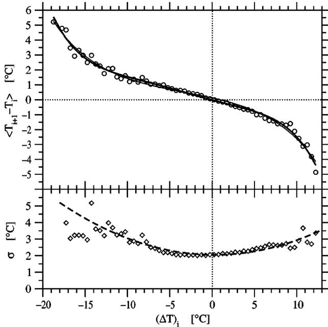
FIG. 3. The components of the empirical “atmospheric response function”  $f(\Delta T)$  for the 16 weather stations in Hungary: the average temperature step  $\langle T_{i+i} - T_i \rangle = f(\Delta T_i) \Delta T_i$  (top) and its standard deviation  $\sigma$  (bottom) as a function of temperature anomaly  $\Delta T_i$ . Cubic (thin line) and fifth-order polynomial (thick line) fits for the temperature steps, as well as a quadratic fit for  $\sigma$  are indicated (see text).
